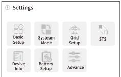
Settings: This interface is used to configure system parameters including Basic Setup, System Mode, Grid Setup, STS, Battery Setup, and Advanced functions, as well as to view fault codes and Device information.
