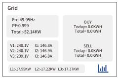
Grid Data: This interface displays Grid voltage, frequency, current, Power, Power Factor, along with energy import from grid, export to grid.
