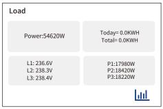
Load Data: This interface displays the load power, phase voltages, as well as today's and cumulative load energy consumption statistics.
