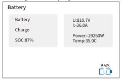
Battery Data: This interface displays the operational data of the battery system connected to the PCS, including charge/discharge status, State of Charge (SOC), voltage, current, power, and temperature information.
